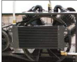
Air cooled after cooler Elite unit
