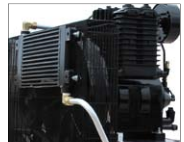
Air cooled after cooler Elite unit
